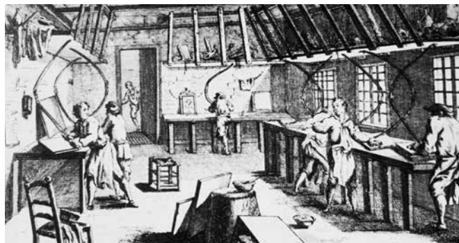
Polishing glass by hand to make mirror plates in an 18th century workshop.
